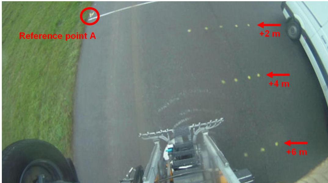
Figure: Video from the top of the spreader showing reference point A and some of the distance markings
